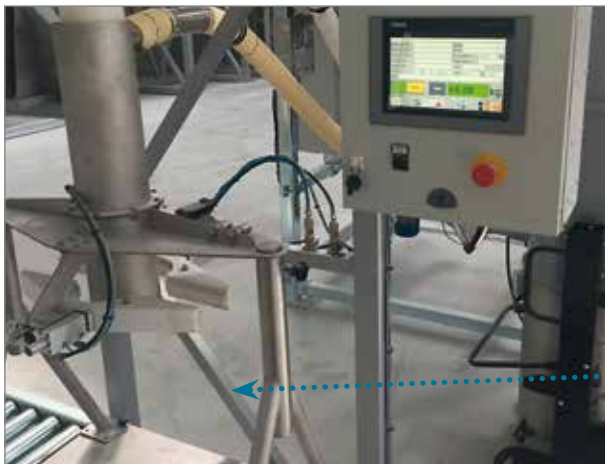
25 kg open mouth bag/box semi-automatic filling including: bulk bag unloading, sieving, metal detecting and dust extraction.
