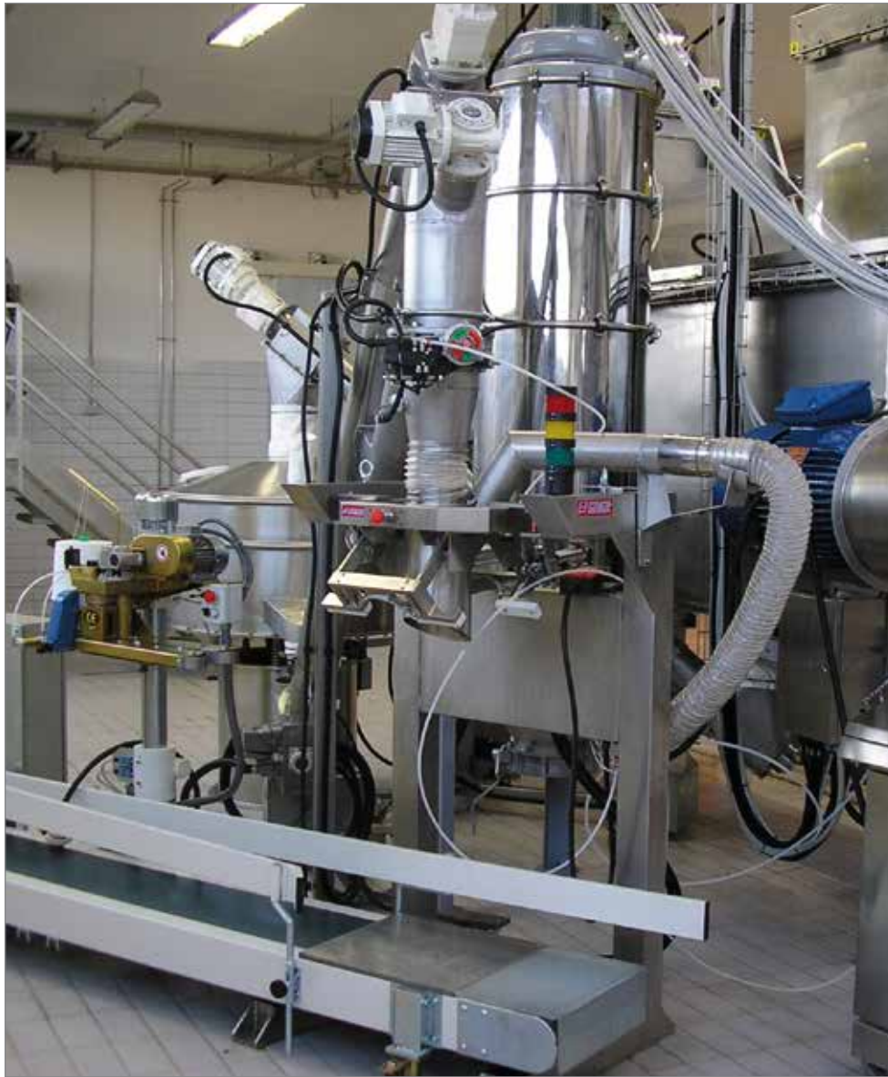
Mix preparation plant including: loading components with powder suction, riddling, batching, bagging and closure
