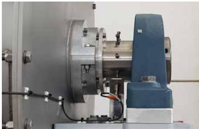
Ball Bearing end support with temperature and speed monitor
