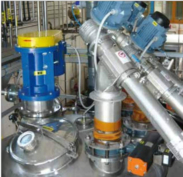
Bag dumping stations complete of screw conveyors for vertical tank feeding with different types of powder
