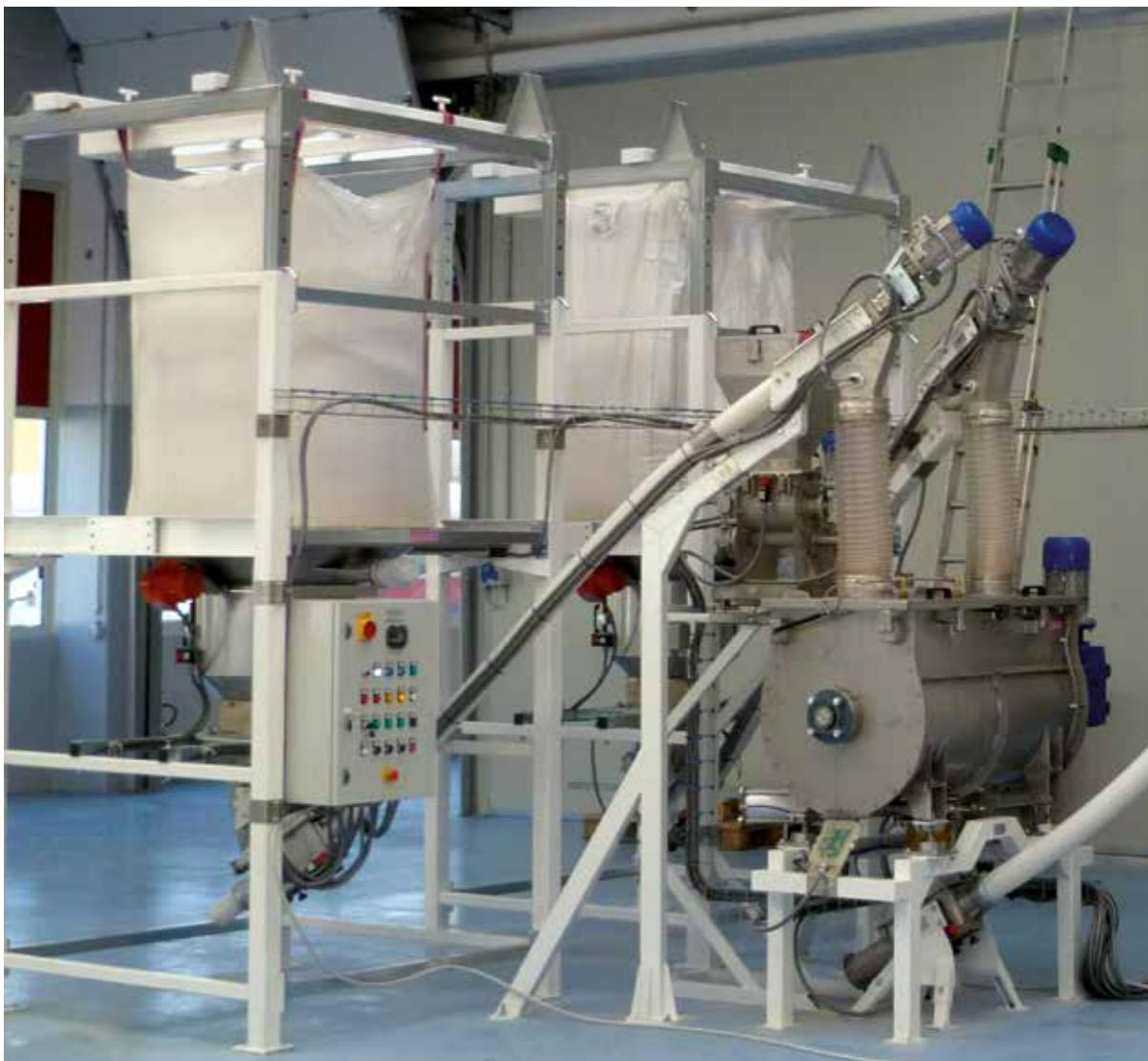
Bulk Bag Unloading with Flexible Screw Conveyors, Dosing, Batch Mixing of three different components and Conveying into buffer silo
