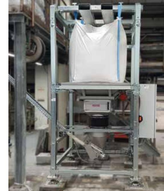
Bulk Bag Unloaders on load cells
