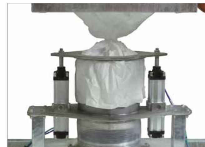
Pneumatic tightening system for dust proof bulk bag discharging
